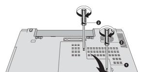
Figure 4-11 Seating the memory module cover
